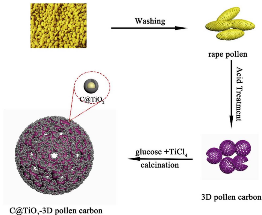
Fig. 8 Schematical illustration of the synthetic process of C@TiO 2 /3D pollen carbon. 114
