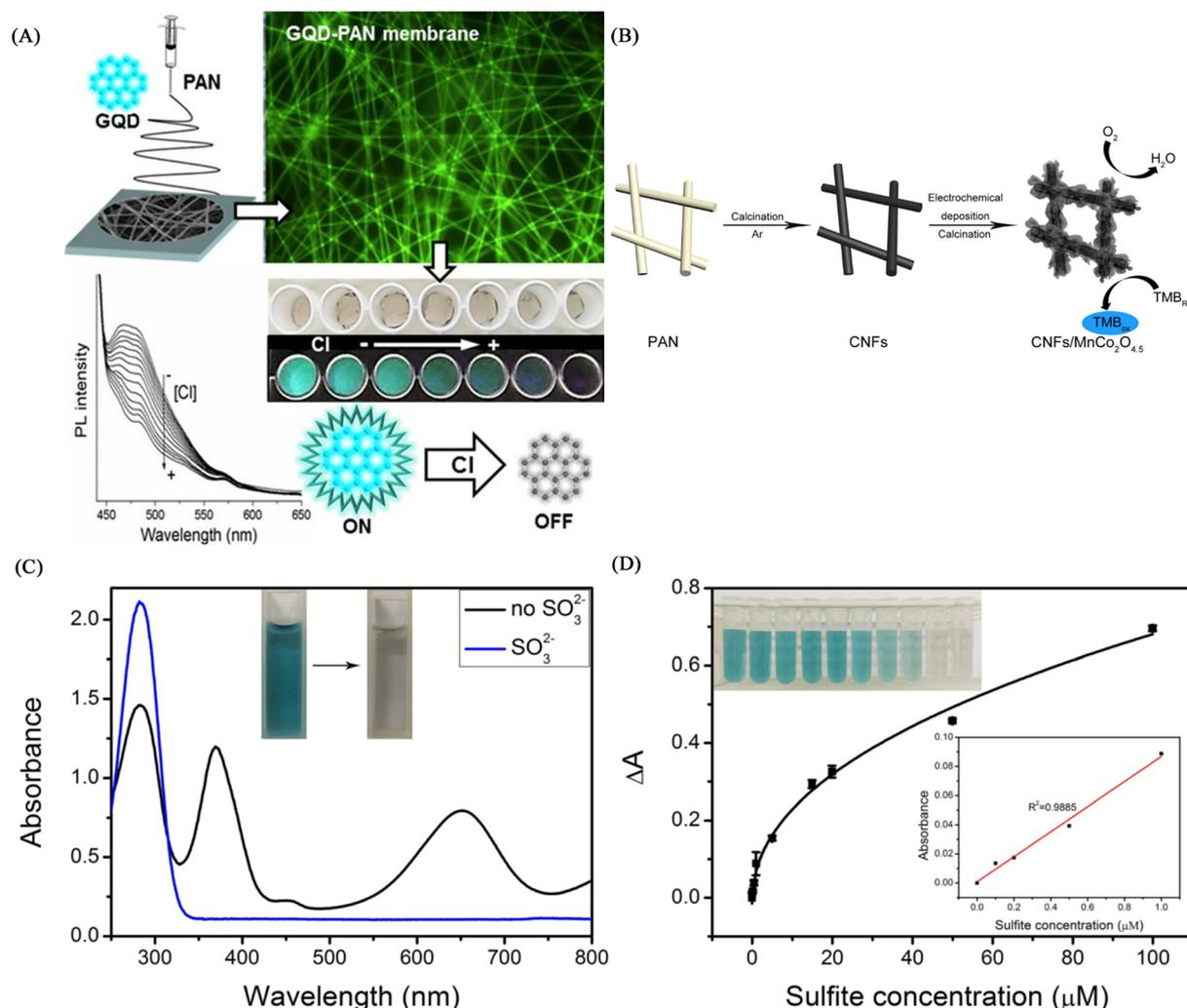
Fig. 21 Fabrication and properties of  $\text{ClO}^-$ ,  $\text{SO}_3^{2-}$ -nanofiber membrane sensors (A) reprinted with permission from ref. 130. Copyright 2018, Elsevier. (B), (C) and (D) reprinted with permission from ref. 131. Copyright 2017, IOP Publishing Ltd.
