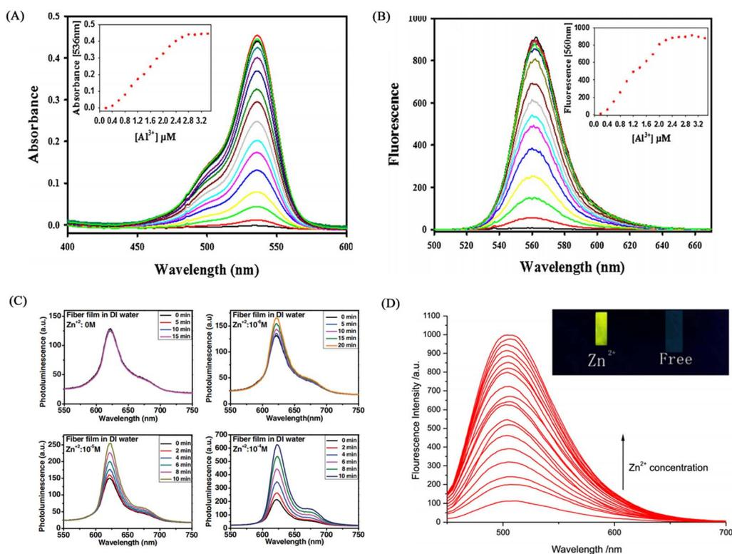
Fig. 18 Sensing properties of  $\text{Zn}^{2+}$ ,  $\text{Al}^{3+}$  sensor. (A) and (B) reprinted with permission from ref. 122. Copyright 2016, Elsevier. (C) Reprinted with permission from ref. 123. Copyright 2013, Wiley-VCH (D) reprinted with permission from ref. 124. Copyright 2017, Chen Zhou *et al.*
