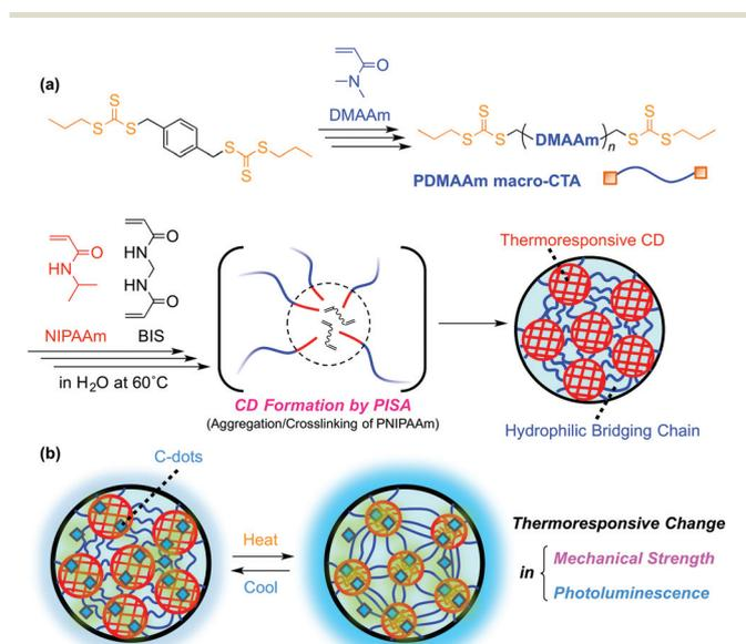
**Fig. 1** (a) Synthesis of a gel having a thermo-responsive CD structure by a PISA process using RAFT polymerization, and (b) thermo-responsive simultaneous change in the mechanical strength and photoluminescence of a gel with a CD structure including C-dots.
