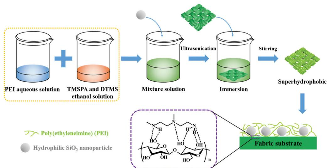
**Scheme 1** Schematic of fabrication of superhydrophobic PEI/TMSPA/SiO<sub>2</sub>/DTMS fabrics.
