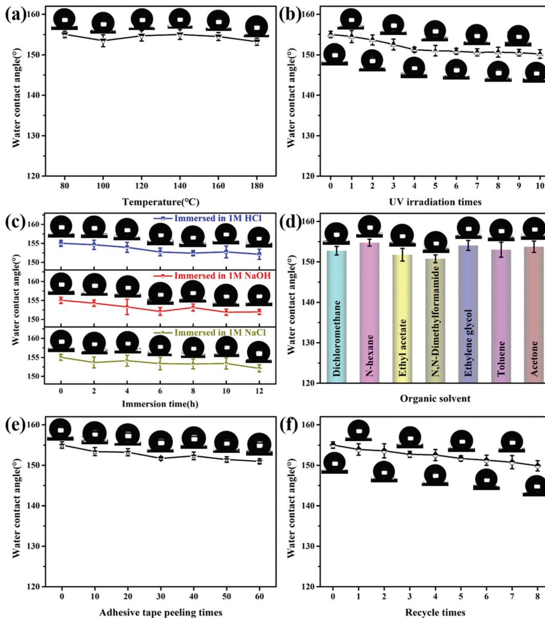
Fig. 6 Variations in the WCA of the PEI/TMSPA/SiO<sub>2</sub>/DTMS fabric after (a) heating at different temperatures for 2 h, (b) UV irradiation with different times, (c) treatment in 1 M NaCl, HCl, and NaOH solutions for different times, (d) immersion in different organic solvents for 24 h, (e) adhesive tape peeling test and (f) washing test.
