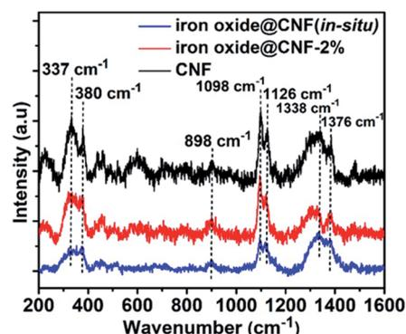
Fig. 4 Raman spectroscopy of iron oxide@CNF nanohybrids.
