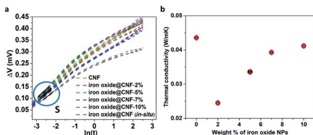
Fig. 7 The graphs showing the changes in the voltage of platinum wire ( $\Delta V$ ) with the logarithm of the time of the measurement  $\ln(t)$  for CNF, iron oxide@CNF nanohybrids by one-pot synthesis (2, 5, 7 and 10 wt% of iron oxide NPs) and iron oxide@CNF nanohybrid by *in situ* synthesis, where  $S$  is the slope of the linear portion.
