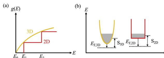
Fig. 15 (a) Arrangements of density-of-states (DOS) and (b) carrier compartments in 3-D bulk materials and 2-D quantum-well materials. The width of the conduction valley in (b) signifies the DOS. Reproduced with permission from ref. 111.
