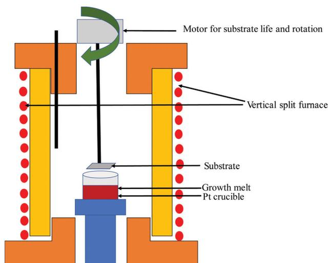
Fig. 13 Representation of the principle of LPE.
