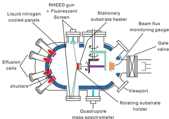
Fig. 14 Schematic of the principle of MBE.
