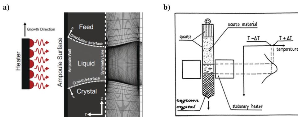
Fig. 12 (a) Left: Representation of the travelling heater method (THM). The heater moves in the upward direction of growth. Right hand side shows the finite element mesh representing 90 axial and radial elements within the liquid zone having a higher density of elements at the boundary. (b) Principle of the travelling heater method. Reproduced with permission from ref. 102 (a) and ref. 102 (b).
