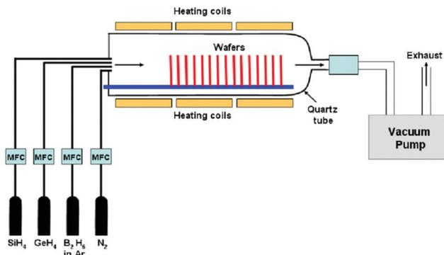
**Fig. 17** Schematic view of the LPCVD system.
