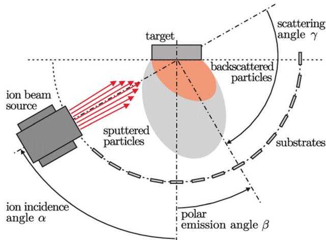
Fig. 19 Representation of the ion-beam sputtering system.
