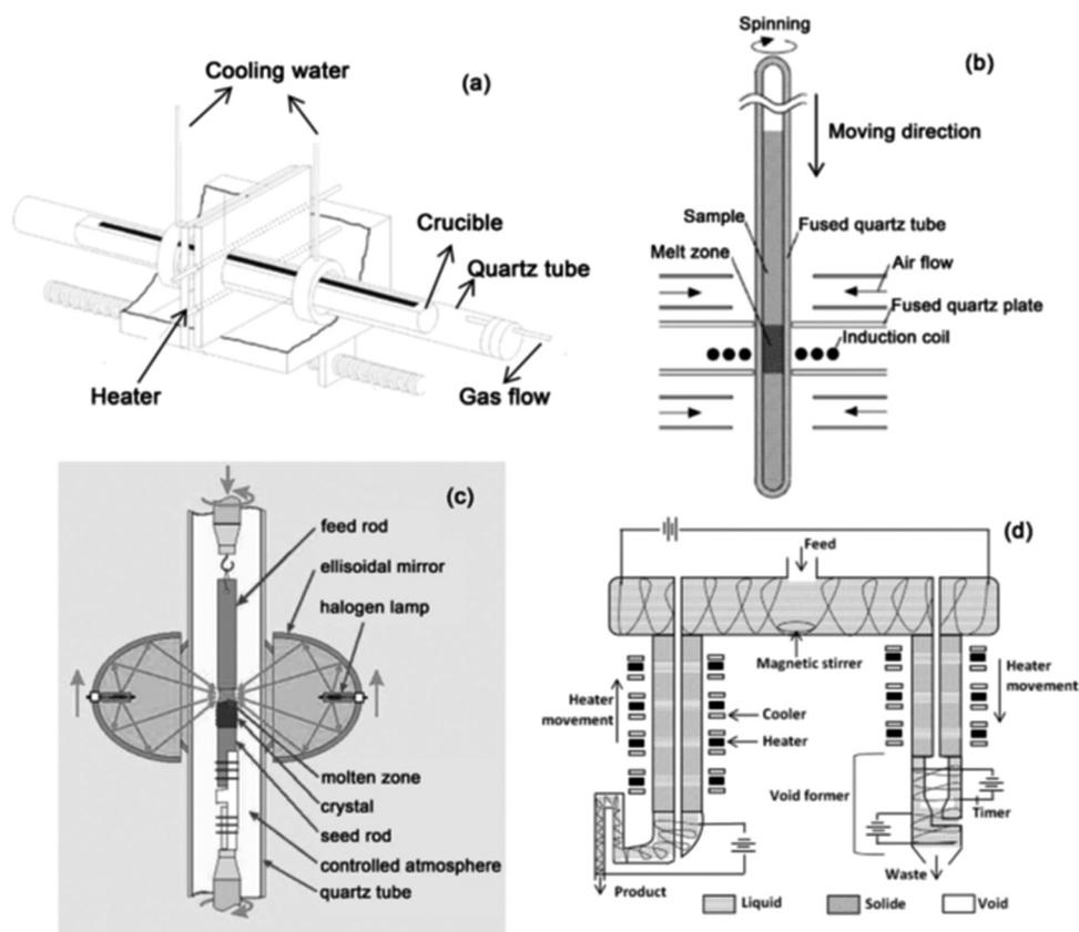
Fig. 7 Arrangement of technologies involved in variable zone refining: (a) horizontal zone refining set up;<sup>79</sup> (b) vertical zone refining set up;<sup>80</sup> (c) floating zone refining set up;<sup>81</sup> (d) continuous zone refining set up,<sup>82</sup> adapted pictures.
