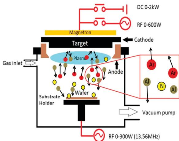
Fig. 18 Schematics of the RF sputtering system.
