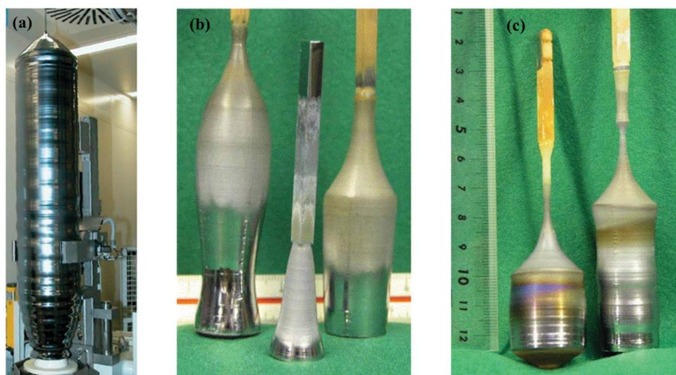
Fig. 5 (a) Silicon crystal having a radius of 150 mm and a weight above 250 kg, grown by the CZ technique (Image courtesy of Siltronic AG4), (b)  $\text{Si}_x\text{Ge}_{1-x}$  alloys developed by the CZ method having [001] oriented Si seed crystal. (c) GeSi boules developed with Dash necking (left) and developed with a Si-Ge seed with identical constituents (right). Reproduced with permission from ref. 53.
