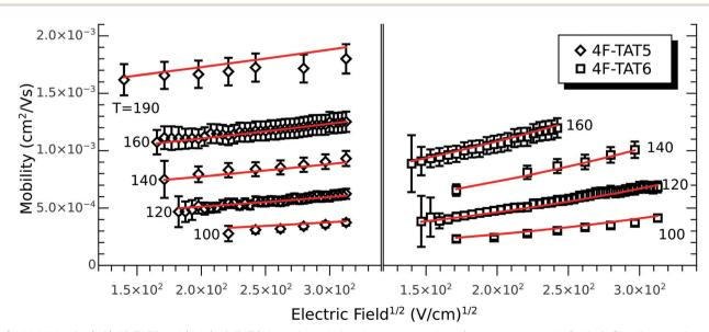
Fig. 8 Mobilities for (left) 4F-TAT5 and (right) 4F-TAT6 throughout their columnar mesophase (temperatures are in Celsius). Gray lines are fits to the model. Removing the tails from the fluorinated ring not only preserves the mesomorphic behavior, but the resulting mobilities remain comparable to their tailed analogues. The large uncertainty at low field reflects the inherent difficulty of extracting a time of flight in this regime.
