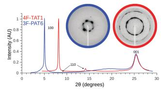
Fig. 5 SAXS diffraction patterns collected from 4F-TAT1 at 220 °C and 3F-PAT6 at 100 °C. A portion of the small angle region is shown in the inset, with an emphasis on the 100 and 110 scattering. 3F-TAT1's lack of long tails results in a much shorter intercolumn spacing and a lack of the broad diffuse scattering associated with the tails. It also results in a greater degree of in-plane order resulting in a number of peaks which are suppressed in 3F-PAT6.
