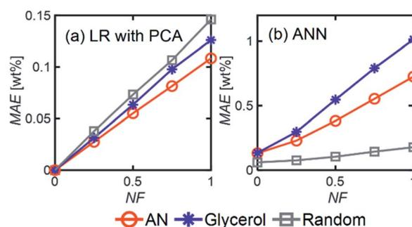
Fig. 8 MAE (averaged over all components) as a function of NF for (a) LR with PCA and (b) ANN models applied to different chemical mixtures and using  $N_{\text{train}} = 400$ . For ANN, 1 hidden layer with 12 neurons was used with an 'relu' activation function and a batch size of 60.
