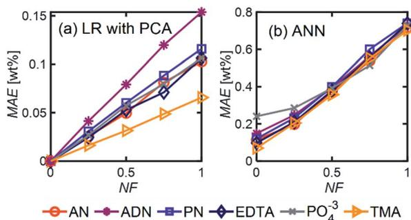
Fig. 6 MAE as a function of NF for (a) LR with PCA and (b) ANN using the model 6-component mixture with  $N_{\text{train}} = 400$ . For ANN, we used 1 hidden layer with 12 neurons, 'relu' activation function, and a batch size of 60.
