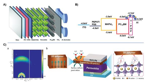
Fig. 8 (A) Device configuration of CON/PEDOT: PSS HTL incorporated PSC. Reproduced with permission from ref. 87. Copyright 2018, Royal Society of Chemistry. (B) Device incorporating T-POP as a secondary ETL. Reproduced with permission from ref. 90. Copyright 2020, Elsevier. (C) GIWAXS plot with device configuration. Reproduced with permission from ref. 92. Copyright 2021, American Chemical Society.
