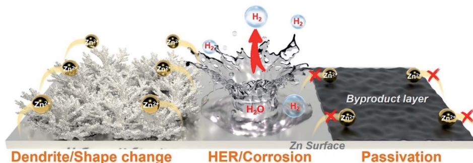
Fig. 13 Schematic diagram showing the dendrite/shape change, HER/corrosion, and passivation problems of Zn NEs.
