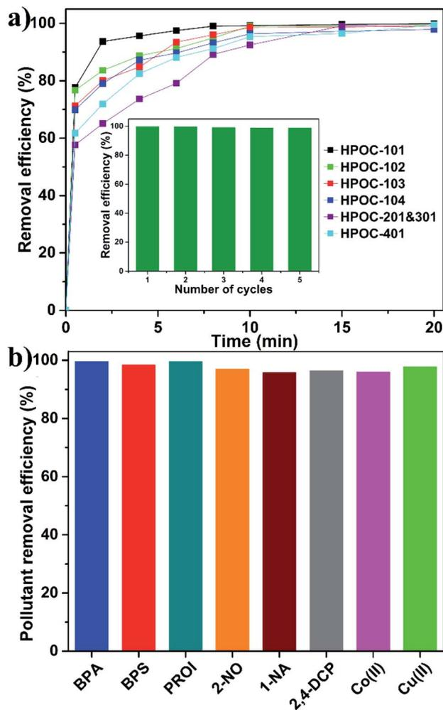
Fig. 5 (a) Time-dependent adsorption of aqueous  $I_3^-$  by hydrazone-linked POCs, inset: the recyclability of HPOC-101 for  $I_3^-$  removal. (b) Percentage removal efficiency of different water pollutants (0.1 mM) by HPOC-101 ( $0.5 \text{ mg mL}^{-1}$ ).
