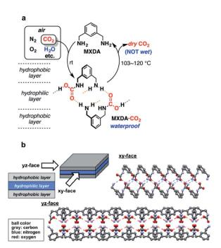
Fig. 4 DAC by crystallization of MXDA. (a) DAC cycle involving atmospheric  $CO_2$  absorption by an aqueous solution of MXDA. (b) Crystal structure of the carbamic acid formed from the reaction of MXDA with  $CO_2$ . Reproduced with permission from ref. 35. Copyright (2017) American Chemical Society.
