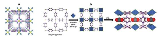
Fig. 1 MOFs/HUMs for DAC by physisorption. (a) Crystal structure of SIFSIX-3-Ni. (b) Crystal structure of NbOFFIVE-1-Ni and binding of CO $_2$  in its pores. Adapted with permission from ref. 20. Copyright (2016) American Chemical Society.
