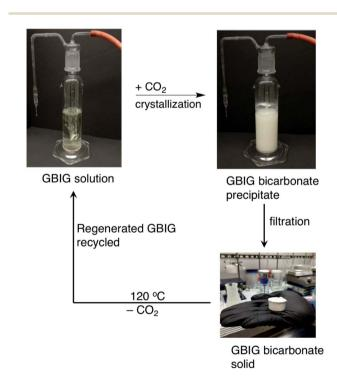
Fig. 7 CO<sub>2</sub> separation via GBIG bicarbonate crystallization. A flue gas simulant (12.8% CO<sub>2</sub>, EPA standard) is bubbled through an aqueous GBIG solution, leading to crystallization of GBIG bicarbonate. The solid is collected by filtration, then heated at 120 °C to release the CO2 and regenerate the GBIG sorbent. The filtrate containing the residual GBIG, and the regenerated GBIG solid are recycled.
