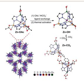
Fig. 3 Crystal structure of a Zn-benzotriazolate MOF functionalized with Zn-OH binding sites and reaction with CO<sub>2</sub>. Reproduced with permission from ref. 32. Copyright (2020) American Chemical Society.
