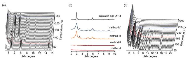
Fig. 5 (a) Variable temperature (VT)-PXRD patterns of the as-formed HOF TolHAT-1. (b) PXRD patterns of activated HOF TolHAT-1aN (N = I - IV) with the simulation pattern of TolHAT-1. (c) VT-PXRD patterns of TolHAT-1aIV from rt to 360 °C. Red line indicates the temperature where the network begins to collapse and blue line corresponds to the temperature where the framework is fully collapsed. The asterisk (\*) denotes a non-identifiable peak appeared for the activated TolHAT samples.
