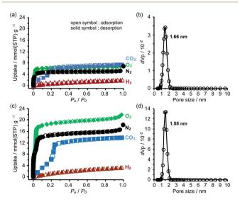
Fig. 7 (a and c) Gas sorption isotherms and (b and d) pore distribution of (a and b) TolHAT-1aIV and (c and d) ThiaHAT-1a. The isotherms were recorded at -196 °C for N<sub>2</sub>, O<sub>2</sub>, and H<sub>2</sub> and at -78 °C for CO<sub>2</sub>. Solid and open symbols denote absorption and desorption processes, respectively
