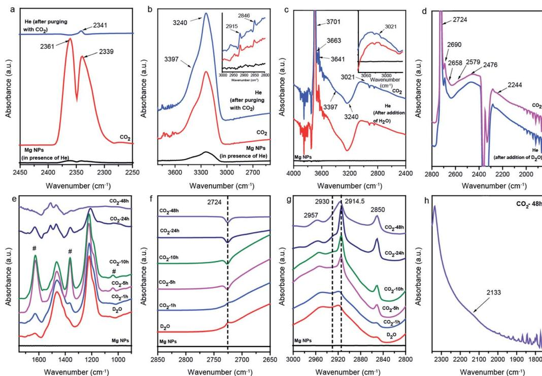
Fig. 3 *In situ* ATR-FTIR spectra: (a and b) in He, CO<sub>2</sub>, and again He, (c) after adding H<sub>2</sub>O to the Mg NPs and subsequently purging with He and CO<sub>2</sub> gas, (d) after adding D<sub>2</sub>O to the Mg NPs and subsequently purging with He and CO<sub>2</sub> gas, and (e–h) after adding D<sub>2</sub>O to the Mg NPs and then purging with CO<sub>2</sub> for 1, 5, 10, 24 and 48 h.
