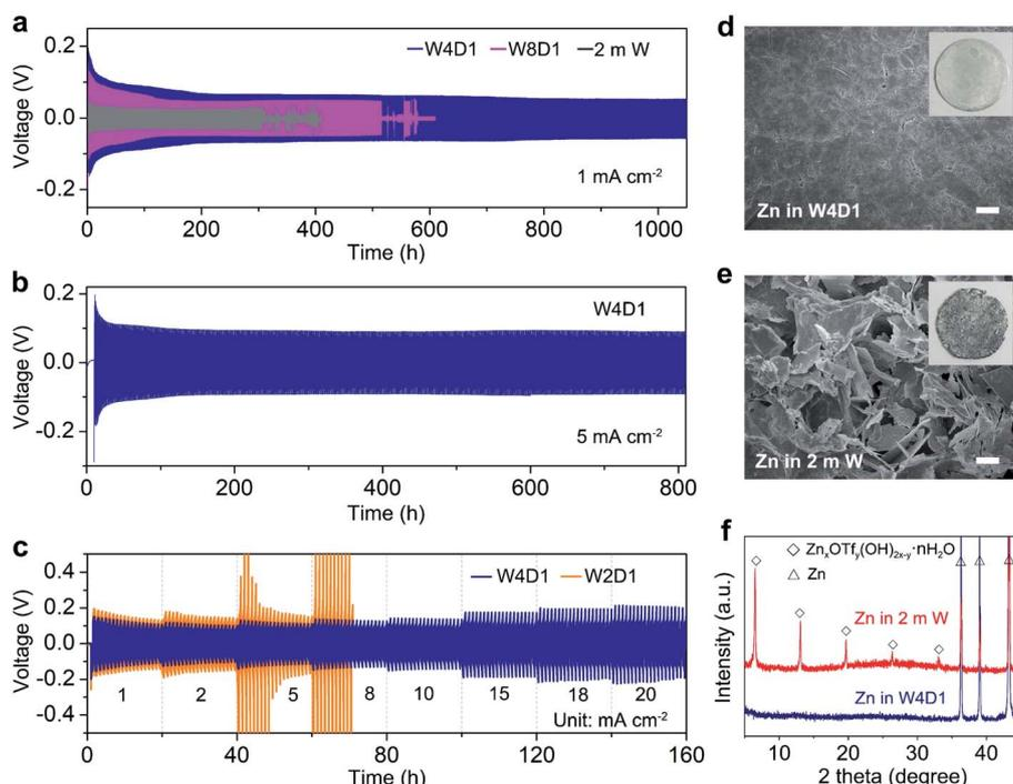
Fig. 4 Electrochemical test and characterization of Zn anodes in Zn/Zn cells. (a) Comparison of voltage profiles in W4D1, W8D1 and 2 m W electrolytes at  $1 \text{ mA cm}^{-2}$ . (b) Cycling performance in the W4D1 electrolyte at  $5 \text{ mA cm}^{-2}$ . (c) Rate capability of Zn/Zn cells with W4D1 and W2D1. (d, e) SEM images (scale bar,  $10 \mu\text{m}$ ) and (f) XRD patterns of Zn anodes after 300 cycles. Insets of (d, e) show the optical images of cycled Zn anodes.
