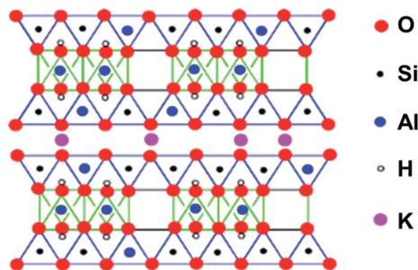
Fig. 7 The structure of a mica, muscovite,  $(\text{KF})_2(\text{Al}_2\text{O}_3)_3(\text{SiO}_2)_6(\text{H}_2\text{O})$ . The space between the layers is occupied only by  $\text{K}^+$  ions. The layer structure facilitates cleavage to produce flat surfaces. Adapted from <https://employees.csbsju.edu/cschaller/PrinciplesChem/network/NWalumina.htm> (accessed 17<sup>th</sup> November 2020), courtesy of Chris Schaller.
