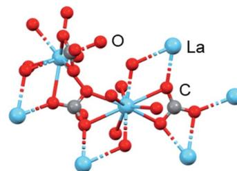
Fig. 10 X-ray crystal structure of  $\text{La}_2(\text{CO}_3)_3 \cdot 8\text{H}_2\text{O}$  (CCDC1599003).  $\text{La}^{3+}$  is 10-coordinate with coordination sites occupied by water, bidentate and monodentate carbonate,  $\text{La}-\text{O}$  bond lengths 2.52–2.74 Å. It is a layer structure with alternate rows of carbonate anions and lanthanide cations. A quarter of the water molecules are unbound and between layers. La, blue; O, red; C, grey.<sup>49</sup> (ICSD-22224).
