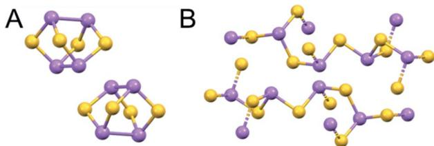
Fig. 3 X-ray crystal structures of naturally-occurring arsenic sulfide minerals (A) Realgar,  $\text{As}_4\text{S}_4$ , (mp-542846) and (B) Arsenicum,  $\text{As}_2\text{S}_3$  (mp-641). As, purple; S, yellow. (mp-542846 DOI: 10.17188/1266759).<sup>15</sup>
