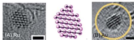
Fig. 4 Ruthenium and gold nanocrystals fabricated on a graphitic support by electron bombardment of  $\text{Ru(II)}$  and  $\text{Au(III)}$  complexes encapsulated in polymer micelles deposited on a lacey carbon EM grid in an aberration-corrected high-resolution transmission electron microscope. Interatomic distances: Ru–Ru 2.48 Å, Au–Au 2.73 Å. Scale bars 1 nm. Adapted from ref. 20 with permission from the Royal Society of Chemistry, copyright 2016.<sup>20</sup>
