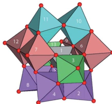
Fig. 15 Structure of  $[Al_{13}O_4(OH)_{24}(H_2O)_{12}]^{7+}$  in its sulfate salt. A central  $Al(O)_4$  unit surrounded by four trimeric groups of edge-shared  $Al(O)_6$  octahedra. Red, O; H atoms omitted. Reprinted with permission from *Inorg. Chem.* 2016, 55, 12270–12280. Copyright 2016 American Chemical Society.<sup>97</sup>
