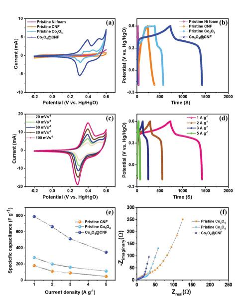
Fig. 5 Comparison of three electrode electrochemical measurements for the pristine  $Co_3O_4$  nanoparticles, pristine CNF and 1D  $Co_3O_4$ @CNF: (a) CV curve at 20 mV s<sup>-1</sup> of scan rate, (b) GCD curve of 1 A g<sup>-1</sup> of current density, (c and d) CV and GCD curves at various scan rates and current densities, (e) specific capacitance and (f) EIS measurement.
