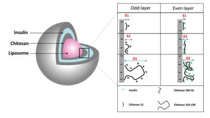
Fig. 1 Schematic drawing of LbL coated liposome and the proposed molecular interaction between insulin and 3 different molecular weights of chitosan.
