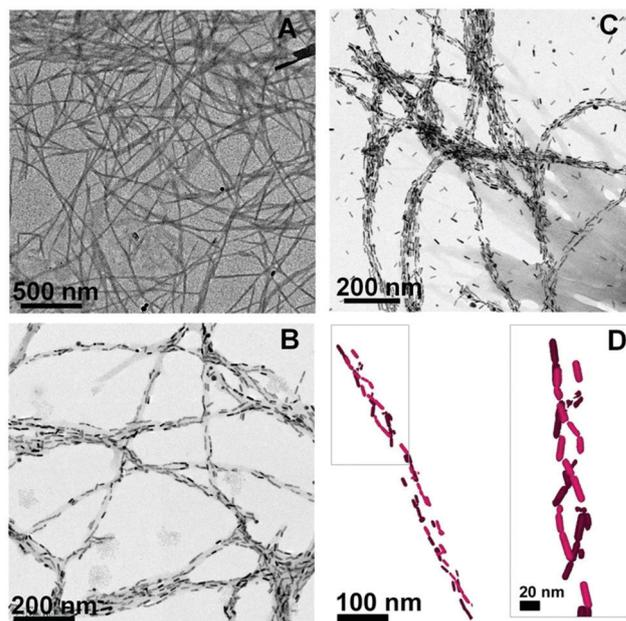
Fig. 19 TEM images of (A)  $\alpha$ -synuclein fibrils, (B)  $\alpha$ -synuclein fibrils mixed with 0.5 nM Au NRs, (C) 2.0 nM Au NRs, and (D) 3D chiral structure of Au NRs. Reprinted with permission.<sup>131</sup> Copyright 2018, the National Academy of Sciences of the United States of America.
