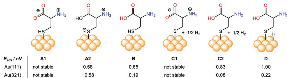
Fig. 2 Pictorial representation and comparison of the simulated surface adsorption energy,  $E_{ads}$  (eV), of different forms of intrinsic L-cysteine amino acid (neutral, ionic, zwitterion) adsorbed on various crystal facets, including achiral Au(111), and chiral Au(321). Reprinted with permission.<sup>70</sup> Copyright 2019, American Chemical Society.
