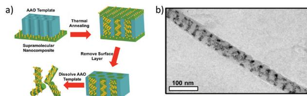
Fig. 17 (a) Schematic diagram showing the steps leading to the formation of Au-nanowires; (b) TEM image of a single-helical nanowire. Reprinted with permission.<sup>120</sup> Copyright 2017, American Chemical Society.
