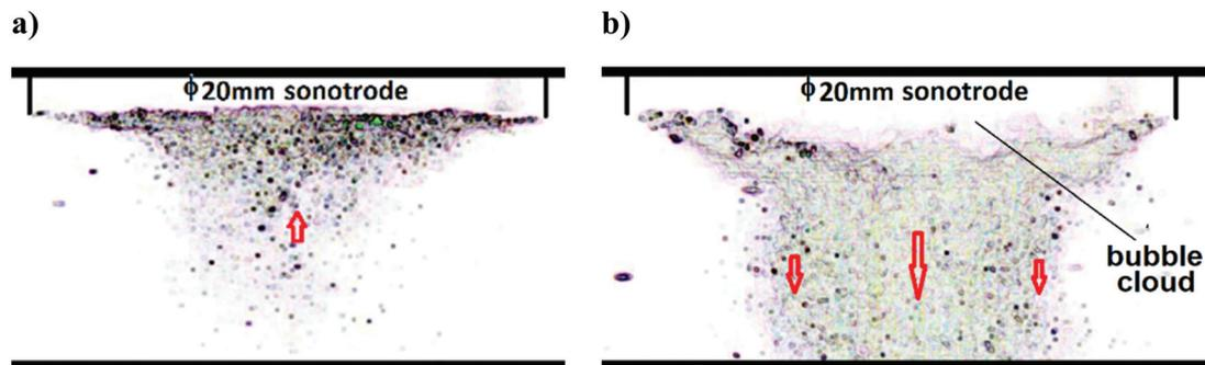
**Fig. 1** High speed camera (20k frames per s) snap shot of cavitation underneath a 20 mm diameter sonotrode at: (a) 20 W cm<sup>-2</sup> and (b) 200 W cm<sup>-2</sup>. The direction of bubble movement is indicated by the arrows. The bubbles close to the axis centre line of the sonotrode cylinder are faster than those away from the centre line.
