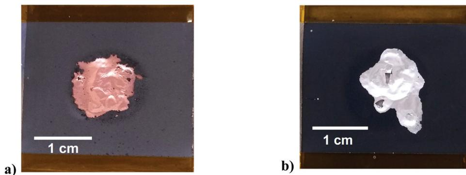
**Fig. 2** Images showing the effect of ultrasound on the front side of a QC reject: (a) anode, and (b) cathode sheets. The anode was delaminated in a solution of 0.05 M citric acid; the cathode was delaminated in a solution of 0.1 M NaOH. The sonotrode was 20 mm in diameter, with 120 W cm<sup>-2</sup> power intensity applied for 3 seconds. Sample size was 3 cm × 3 cm, placed 2.5 mm away from the sonotrode.
