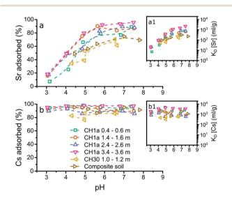
Fig. 2 Graphical representation of the results from the aqueous analyses from the adsorption experiments to the composite clayey soil and the LFLS core samples (initial concentrations of 20 Bq ml $^{-1}$  Sr-85 and Cs-137) with the % of Sr (a) or Cs (b) adsorbed plotted against pH, and the respective  $K_{\rm D}$  values (a1 and b1). The legend represents the location  $^{46}$  and depth of the LFLS core samples used in the adsorption experiments.
