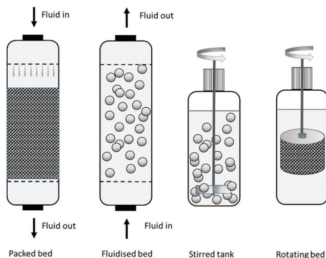
Fig. 8 Reactor design.
