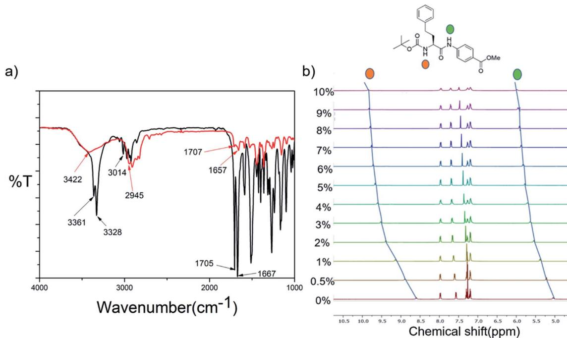
Fig. 5 (a) Superimposed FT-IR spectra of P2 in powder (black) and xerogel (red) states. (b) Stacked NH region of the  $^1\text{H}$  NMR spectra obtained upon addition of increasing amounts of DMSO- $\text{d}_6$  to the  $\text{CDCl}_3$  solution of P2.
