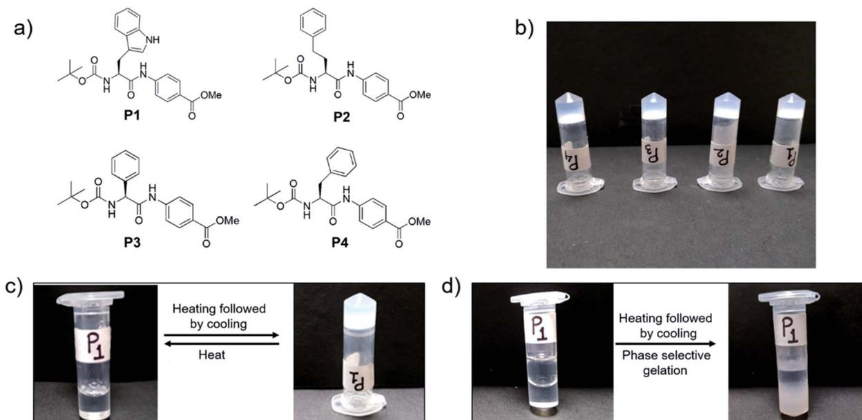
Fig. 1 (a) Chemical structures of LMWG **P1**–**P4**, (b) gels formed in 1,2-DCB by **P1**–**P4** (c) thermoreversibility of the organogel formed by **P1** in 1,2-DCB and (d) phase selective gelation of **P1** in 1,2-DCB in the presence of water.
