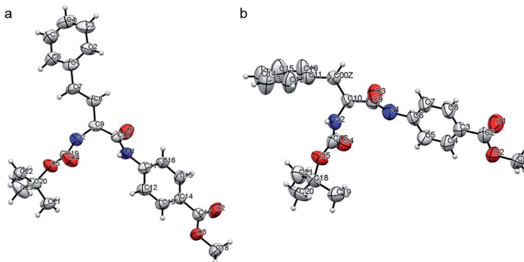
Fig. 6 An ORTEP diagram for peptides (a) P2 and (b) P4, with an ellipsoid of 50% probability, as obtained in the crystals grown from the slow evaporation of MeOH–H<sub>2</sub>O.
