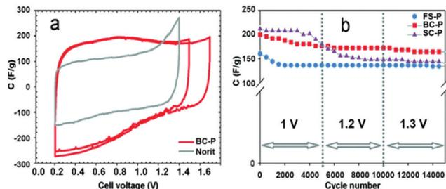
Fig. 18 (a) Cyclic voltammograms of BC-P recorded at  $5 \text{ mV s}^{-1}$  and the cell voltage of 1.3 and 1.5 V compared with Norit at 1.2 V. (b) Galvanostatic cycling at the current load of  $5 \text{ A g}^{-1}$  and cell voltage of 1, 1.2, and 1.3 V. Reproduced with permission from ref. 125. Copyright 2009 American Chemical Society.
