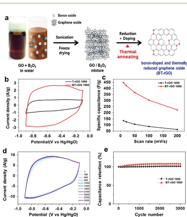
Fig. 20 (a) Schematic illustration of the preparation of BT-rGO. (b) CV curves at a scan rate of 10 mV s<sup>-1</sup>. (c) Specific capacitances as a function of scan rate. (d) CV curves for 3000 cycles at a scan rate of 50 mV s<sup>-1</sup>. (e) Capacitance retentions as a function of cycle number of T-rGO and BT-rGO electrodes. Reproduced with permission from ref. 138. Copyright 2015 Springer Nature.
