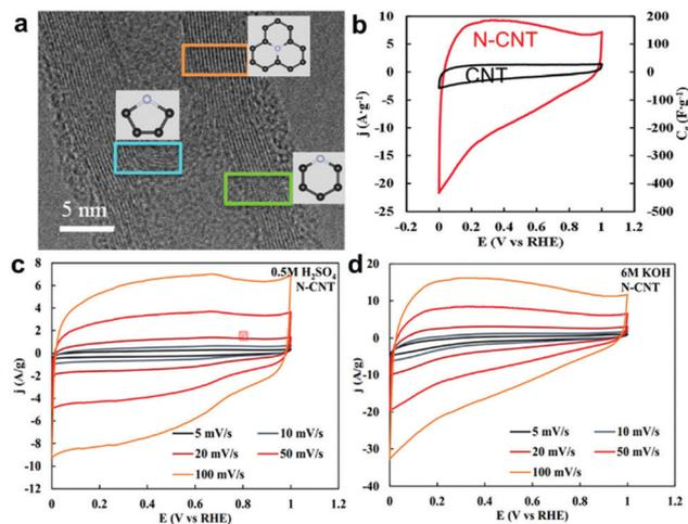
Fig. 17 (a) TEM images of the N-CNTs and three kinds of nitrogen configurations. (b) Cyclic voltammograms of N-CNT (red line) and CNT (black line) electrodes in 6 M KOH solutions at 50 mV s<sup>-1</sup>. Cyclic voltammetry of N-CNT at different scan rates (c) in 0.5 M H<sub>2</sub>SO<sub>4</sub> and (d) in 6 M KOH. Reproduced with permission from ref. 115. Copyright 2014 The Royal Society of Chemistry.
