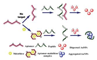
**Fig. 7** Schematic illustration of colorimetric assay for malathion based on aptamer, cationic peptide and AuNPs. The AuNPs remain red in the absence of malathion due to the interaction of aptamer and peptide, whereas in the presence of malathion, the color of the particles becomes blue as the aptamer binds to malathion and the peptide is free to aggregate the particles. Image reprinted from ref. 91 with permission. Copyright 2016 Elsevier.
