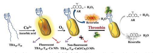
Fig. 4 Schematic representation of the preparation of Apt-CuO/Cu<sub>2</sub>O NPs exhibiting peroxidase-like catalytic activity, and their application in the determination of thrombin based on inhibition of its enzymatic activity using  $H_2O_2/AR$  redox system as fluorescent transducer. Image reprinted from ref. 75 with permission. Copyright 2015 Elsevier.
