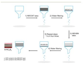
Fig. 1 Schematic illustration of the preparation process of RCB composites with a layered structure. The picture shows the 8-RC<sub>8</sub>B<sub>8</sub> composite. The same process was adopted to produce some layered structures by using graphene as an alternative to carbon nanotubes.
