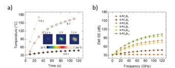
Fig. 5 (a) The time-dependent temperature profiles of  $8\text{-RC}_4B_8$  composites for the different input voltages. The inset picture is an IR image of the  $8\text{-RC}_4B_8$  composite surface after inputting voltage for 30 s. (b) The effect of filler content on the electro heating behaviour with an input voltage of 2.5 V.
