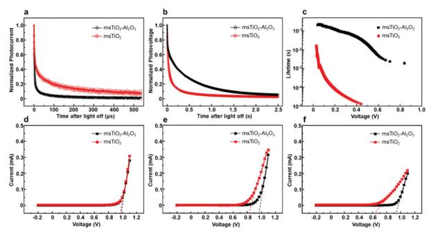
Fig. 5 Transient (a) photo-current and (b) photo-voltage decay of the PSCs based on different mesoporous scaffolds after storing for 12 weeks in ambient air at >65% relative humidity. (c) Electron lifetimes for the above PSC devices. (d) -(f) J-V curves under the dark condition of different PSCs after storing for 0 week, 6 weeks, and 12 weeks, respectively.
