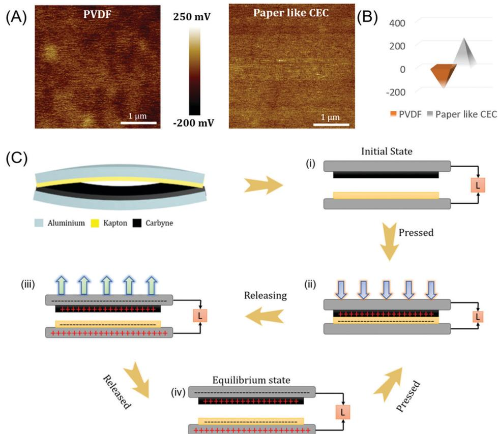
Fig. 4 (A) Surface potential mapping of the PVDF and P-CEC films analyzed *via* KPFM measurement, (B) plot of the change in surface potential before and after the exclusion of halogen, and (C) working mechanism of the P-CEC TENG in the vertical contact-separation mode.
