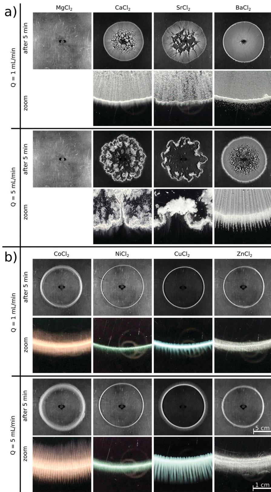
**Fig. 1** Grayscale images of the precipitation patterns observed in the different chemical systems with direct injection for various flow rates 5 minutes after the end of the injection ( $V_{\text{max}} = 5$  mL). Close-ups of the macroscopic patterns shown in real color.
