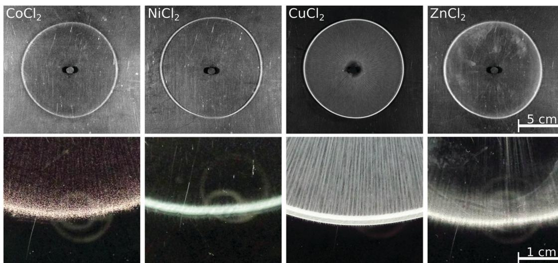
Fig. 3 Grayscale images of the precipitation patterns observed in the different chemical systems with reverse injection at  $Q = 1 \text{ mL min}^{-1}$  flow rate 5 minutes after the end of the injection ( $V_{\text{max}} = 5 \text{ mL}$ ). Close-ups of the macroscopic patterns shown in real color.
