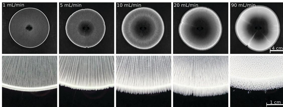
Fig. 4 Grayscale images of the  $\text{Cu}(\text{COO})_{2(s)}$  patterns observed with reverse injection at various flow rates 5 minutes after the end of the injection ( $V_{\text{max}} = 5 \text{ mL}$ ). Close-ups of the macroscopic patterns are also shown.
