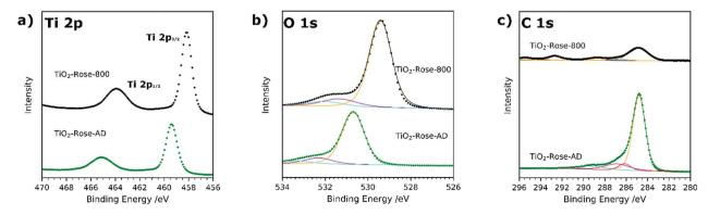
Fig. 5 XPS spectra of (a) Ti 2p, (b) O 1s and (c) C 1s of TiO<sub>2</sub>-Rose-800 and TiO<sub>2</sub>-Rose-AD. Scattered points correspond to raw data acquired in the measurements and solid lines to the fitted values.
