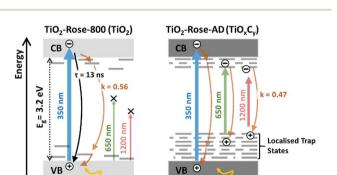
Fig. 9 Schematic diagram representing the difference in the photogenerated charge carrier dynamics for TiO2-Rose-800 and TiO2-Rose-AD when excited with 350, 650 or 1200 nm laser pulses with a photon flux of  $3.97 \times 10^{13}$ ,  $2.01 \times 10^{14}$  and  $1.22 \times 10^{14}$  photons cm<sup>-</sup> pulse<sup>-1</sup>, respectively
