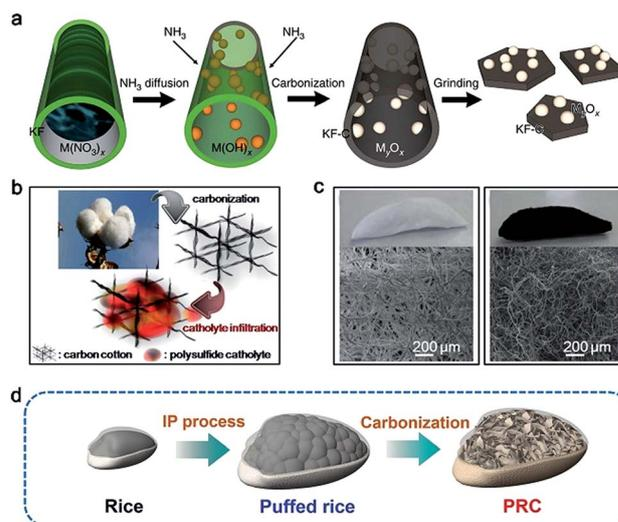
Fig. 2 (a) Fabrication diagram of  $M_xO_y/C$  composites. Reproduced with permission.<sup>12</sup> Copyright 2016, Nature publishing group. (b) Schematic of the fabrication process of carbonized cotton. (c) Digital and SEM images of cotton and carbonized cotton. Reproduced with permission.<sup>50</sup> Copyright 2016, American Chemical Society. (d) Schematic illustration of PRC. Reproduced with permission.<sup>54</sup> Copyright 2017, Wiley-VCH.
