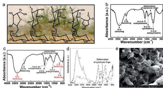
Fig. 6 (a) Chemical structure of GA with the background of *Acacia senegal*. (b) FTIR spectra of GA. (c) FTIR spectroscopy of a mixture of GA-polysulfide composites. (a-c) Reproduced with permission.<sup>26</sup> Copyright 2015, Wiley-VCH. (d) FTIR spectroscopy spectra of (1) Na-alginate and (2) Na-alginate sulfur electrodes. (e) SEM images of the Na-alginate sulfur cathode. (d and e) Reproduced with permission.<sup>86</sup> Copyright 2013, Elsevier.
