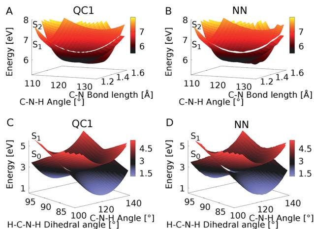
Fig. 5 Potential energy scans around the minimum energy conical intersections obtained with QC1 of the  $S_2$  and  $S_1$  states (A and B) and  $S_1$  and  $S_0$  states (C and D). Panels A and C show the PESs calculated with QC1, while panels B and D illustrate NN potentials. See the caption of Fig. S7 in the ESI† for clarification of the dihedral angle.
