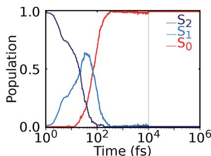
Fig. 4 Nonadiabatic molecular dynamics simulations using deep NNs for one nanosecond. After excitation to the  $S_2$  state, ultrafast internal conversion to the  $S_1$  state takes place, followed by recovery of the  $S_0$  state within 300 fs. Until 10 ps, an ensemble of 200 trajectories is analyzed, followed by the population averaged from 2 trajectories.
