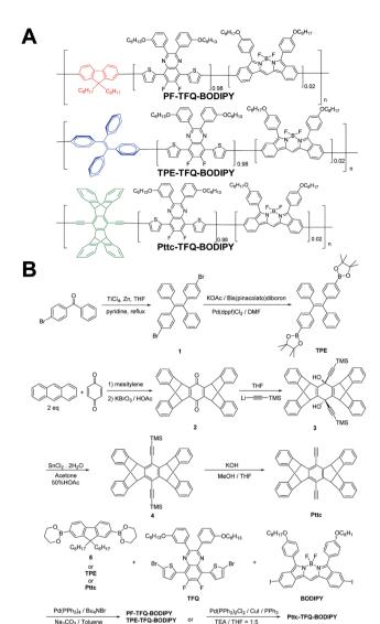
Scheme 1 Schematic showing (A) the chemical structures of three NIR semiconducting polymers with different donors and (B) their synthetic routes
