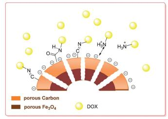
Scheme 4 Schematic of the preparation and drug loading of the porous hollow Fe<sub>3</sub>O<sub>4</sub>@C nanocapsules.<sup>79</sup>
