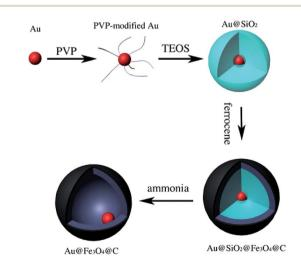
Fig. 8 Schematic of the preparation procedure of yolk-type Au@Fe3O4@C.80
