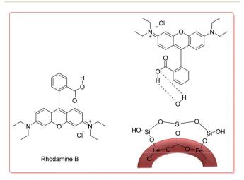
Scheme 1 The structures of RhB and RhB-γ-Fe<sub>2</sub>O<sub>3</sub>@SiO<sub>2</sub>.<sup>48</sup>
