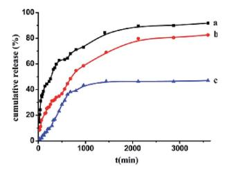
Fig. 4 Cumulative ibuprofen release rates from the drug-adsorbed super paramagnetic polyelectrolyte hybrid hollow microspheres (CS/Fe $_3$ O $_4$ -CA) $_3$ -CS in pH 7.4 phosphate buffer at 37 °C (a) and from the biocompatible (CS/Fe $_3$ O $_4$ -CA) $_3$ -CS-NH-CH $_2$ -PEG hollow microspheres in phosphate buffer at pH 7.4 (b) or 1.8 (c) at 37 °C, respectively.<sup>57</sup>
