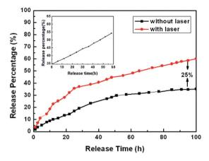
Fig. 9 In vitro release profiles of DOX-Au@Fe $_3O_4$ @C nanoparticles with (red) and without (black) laser irradiation for 100 h. Inset: further DOX release (black) on the balance for another 60 h with laser radiation.
