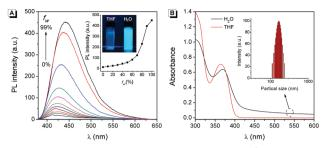
Fig. 1 (A) Fluorescence emission spectra of 50  $\mu$ mol L<sup>-1</sup> 2 in water/THF mixtures with different  $f_{w}$ . Inset: Fluorescence intensity of 2 at 445 nm as a function of  $f_{\rm w}$  and fluorescence photograph of  ${\bf 2}$  in THF and  ${\rm H_2O}$ (99% water/THF (v/v) solution). (B) Absorption spectra of 50  $\mu$ mol L $^{-1}$  2 in THF and H<sub>2</sub>O. Inset: DLS results of 2 in H<sub>2</sub>O.
