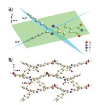
Fig. 2 Crystal structure of 2. (A) The dihedral angles between the conjugate rigid planes. (B) The packing of 2 in the crystal and the minimum distance between the adjacent conjugate planes.
