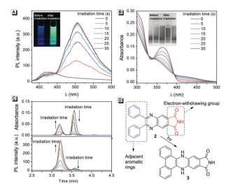
Fig. 3 (A) Fluorescence spectra and (B) absorption spectra of 10  $\mu$ mol L $^{-1}$ 2 in THF before and after UV light irradiation. (C) HPLC analysis of the photoconversion of 10  $\mu$ mol L<sup>-1</sup> 2 to 3 under UV light irradiation for different times. (D) Proposed mechanism for the photo-response performance of 2 upon UV light irradiation.
