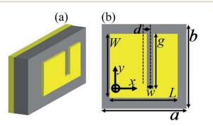
Fig. 1 Three-dimensional structure drawing (a) and front view (b) of the suggested broadband PMA.
