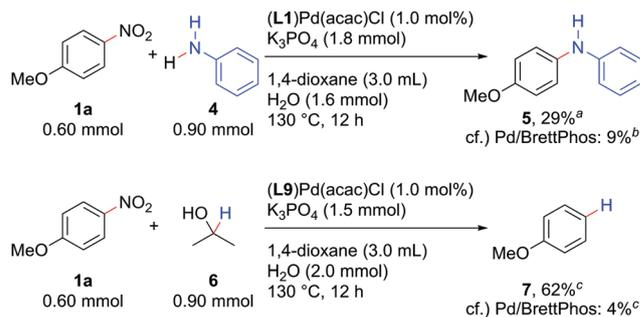
**Scheme 4** The Buchwald–Hartwig amination and reductive denitration of nitroarenes. <sup>a</sup>Isolated yield. <sup>b</sup>NMR yield determined using 1,3,5-trimethoxybenzene as an internal standard. <sup>c</sup>GC yields determined using *n*-C<sub>13</sub>H<sub>28</sub> as an internal standard.
