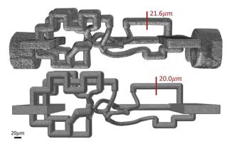
Fig. 9 3D volume rendering of a fabricated microvascular network (top) and its digital mask (bottom) shows a close agreement in overall architecture and channel diameters between them. SB =  $20~\mu m$ .
