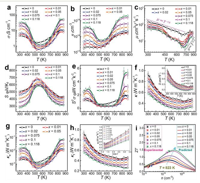
Fig. 6 Plots of measured properties of (a) T-dependent  $\sigma$ ; (b) T-dependent n; (c) T-dependent  $\mu$ ; (d) T-dependent S; (e) T-dependent S (e) T-dependent S (ii) T-dependent S with inset of T-dependent S with inset of T-dependent S with predicted plots for our Cu-doped SnSe pellets.
