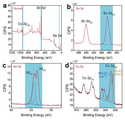
(a) Survey scan of XPS spectra for synthesized products with x = 0.118. High-resolution scans of XPS spectra for (b) Sn 3d, (c) Se 3d, and (d) Fig. 5 Cu 2p.
