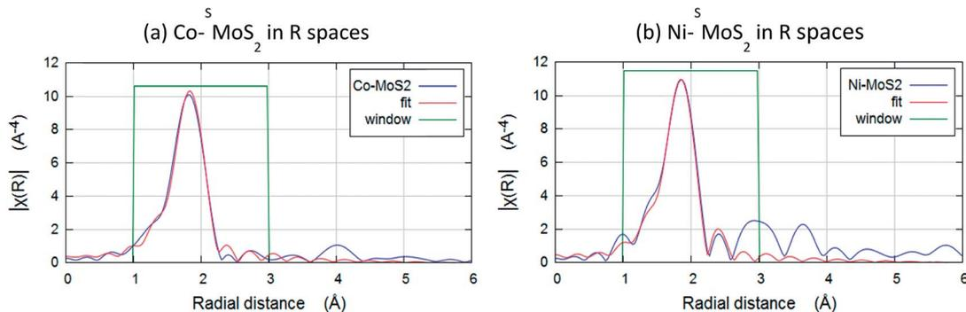
Fig. 6 Fourier transforms of the  $k^3$ -weighted Co and Ni K-edge of extended X-ray absorption fine structure spectroscopy (EXAFS) spectra of (a)  $\text{Co-SMoS}_2$  and (b)  $\text{Ni-SMoS}_2$ .
