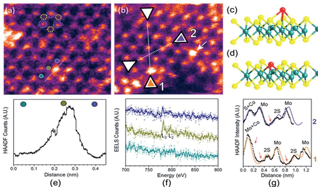
Fig. 3 (a) and (b) HAADF-STEM images of  $Co-SMoS_2$ .<sup>29</sup> Simultaneous acquisition of (c) Co at the Mo-atop site model and (d) Co at the S vacancy site model (e) ADF and (f) EELS acquired along the line in (a). (g) ADF intensity line profiles taken along the numbered lines 1 and 2 shown in (b) ( $\llcorner 110$ ) direction). The red arrows in the plot indicate sample drift during image acquisition.
