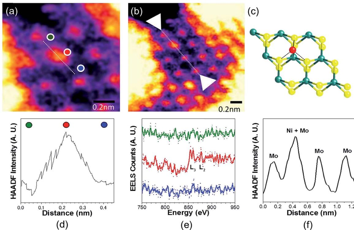
Fig. 4 (a) and (b) HAADF-STEM images of Ni-<sup>5</sup>MoS<sub>2</sub>. (c) Ni at Mo-atop site model (d) ADF and (e) EELS acquired along the line in b. (f) ADF intensity line profile acquired along the line in b of the Mo sites in  $\langle 100 \rangle$  direction.
