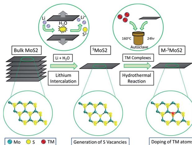
Fig. 1 Synthesis of single-layered MoS<sub>2</sub> (<sup>S</sup>MoS<sub>2</sub>) and single transition-metal (TM) atom doped <sup>F</sup>MoS<sub>2</sub>/<sup>S</sup>MoS<sub>2</sub>SO<sub>4</sub><sup>2-</sup> groups.
