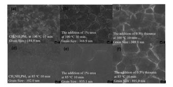
Fig. 2 FE-SEM images of MAPbl $_3$  perovskite thin films under different conditions (a) MAPbl $_3$ , (b) 1% urea, (c) 0.5% thiourea at 100 °C for 10 min, respectively; (d) MAPbl $_3$ , (e) 1% urea, (f) 0.5% thiourea at 85 °C for 10 min, respectively, (scale bar 100 nm).
