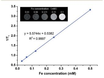
Fig. 9 The *in vitro* MR imaging ability of DOX@ZIF-HA. The linear fitting of  $1/T_1$  as a function of Fe concentration. The inset pictures represent the corresponding  $T_1$ -weighted MR images of DOX@ZIF-HA at different Fe concentrations.
