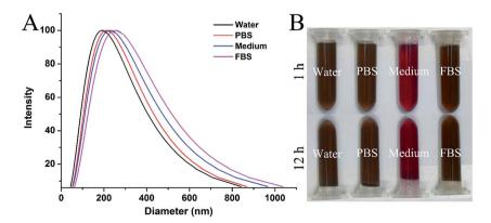
Fig. 3 (A) The size distribution of DOX@ZIF-HA dispersed in different media, as measured by DLS. (B) Photographs of different DOX@ZIF-HA dispersions stored under ambient conditions for 1 h and 12 h.
