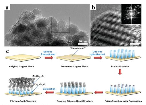
Fig. 11 (a) TEM and (b) HRTEM images of Fe-doped ZnO nanoparticles, inset in panel (b) showing the corresponding FT. Reproduced with permission. 132  $Copyright\ 2013,\ American\ Chemical\ Society.\ (c)\ Preparation\ procedure\ of\ Zn_xCo_{3-x}O_4@Zn_{1-y}Co_yO\ binary\ nanoarrays.\ Reproduced\ with\ permission.^{133}$ Copyright 2016, American Chemical Society
