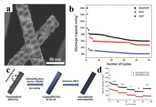
Fig. 6 (a) TEM image of ZnO/CNT composites; (b) cycling performances of bare CNTs, ZnO, and ZnO/CNT electrodes. Reproduced with permission.<sup>79</sup> Copyright 2013, Springer. (c) Schematic illustration of facile sol-gel synthesis of nanocomposite anodes; (d) the rate capabilities of the ZnO/MWCNT buckypaper nanocomposite anodes. Reproduced with permission.<sup>81</sup> Copyright 2015, Elsevier.
