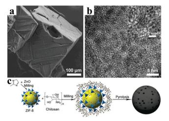
Fig. 7 (a) SEM image and (b) TEM image of ZnO QDs@porous carbon. Reproduced with permission. 93 Copyright 2013, American Chemical Society. (c) Synthetic route of ZIF-8@chitosan-800N. Reproduced with permission. 94 Copyright 2014, Royal Society of Chemistry.
