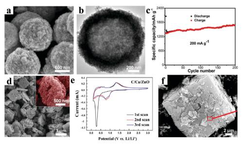
Fig. 10 (a) SEM and (b) TEM images of sandwich-like Ag-C@ZnO-C@Ag-C hybrid hollow microspheres; (c) cycling performances at 0.2 A  $g^{-1}$ . Reproduced with permission. 129 Copyright 2015, American Chemical Society. (d) SEM image and (e) CV curves of the C/Cu/ZnO hybrids. Reproduced with permission.<sup>130</sup> Copyright 2014, American Chemical Society. (f) SEM image of the CZO@C. Reproduced with permission.<sup>131</sup> Copyright 2014, American Chemical Society.
