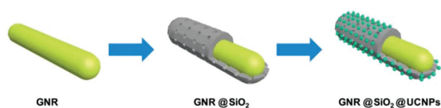
Scheme 1 Schematic illustration of the synthetic procedure for the preparation of the GNR@SiO 2 @UCNPs nanocomposite.
