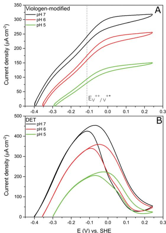
Fig. 7 Comparison of cyclic voltammograms of *DdHydAB* immobilized on viologen-modified GCE (A) and in a DET system on a PGE (B) at three different pH values in an aqueous buffer. Conditions:  $5 \text{ mV s}^{-1}$ ,  $25^\circ\text{C}$ , 1000 rpm, 100%  $H_2$ .
