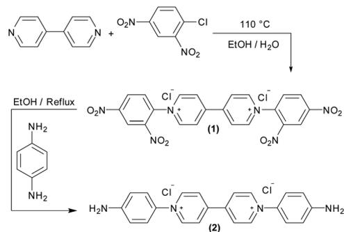
**Scheme 1** Synthesis of the viologen derivative 1,1'-bis(4-amino-phenyl)-[4,4'-bipyridine]-1,1'-diium chloride (2).
