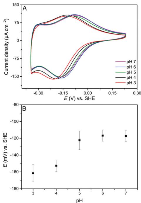
Fig. 2 Redox potential at different pH values. (A) CVs of a viologen-modified GCE at different pH values. (B) Viologen redox potential vs. pH ( $n = 3$ ). Conditions: aqueous mix buffer, 100 mV s<sup>–1</sup>, 25 °C, N<sub>2</sub>.
