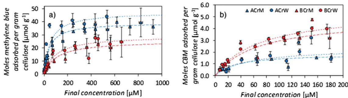
Fig. 3 (a) Methylene blue adsorption isotherms on regenerated cellulose scaffolds, (b)  $ThCBM_{CBHI}$  adsorption isotherms on regenerated cellulose scaffolds. Error bars  $\pm 1$  standard error. Whilst a greater surface area is accessible to methylene blue in  $\alpha$ -cellulose samples, a greater area is accessible to  $ThCBM_{CBHI}$  in bacterial cellulose samples. Water regenerated samples have a greater accessible area in all cases.
