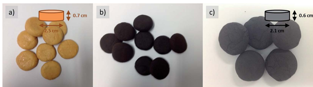
Fig. 4 Doughs obtained from glucose-urea-ZnCl 2 /H 2 O + 39% cellulose before and after baking (a) viscoelastic pellets of the dough, (b) pellets pre-baked at 100 °C for 3 hours, the green body, and (c) carbonaceous pellets made at 500 °C in nitrogen atmosphere.
