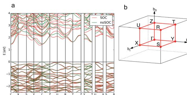
Fig. 11 Calculated band structure of bournonite ( $\text{CuPbSbS}_3$ ) showing the result without the inclusion of spin-orbit coupling (SOC) in green and the calculation including SOC in red (a) and the reciprocal space  $k$ -path for the structure determined by the Aflow-online utility<sup>74</sup> (b).
