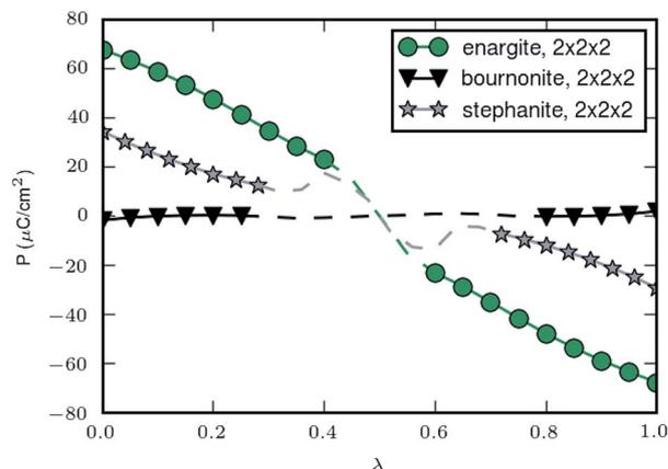
Fig. 14 Spontaneous polarisation along a path connecting the structures with  $+P_s$  and  $-P_s$  for enargite ( $\text{Cu}_3\text{AsS}_4$ ), stephanite ( $\text{Ag}_5\text{SbS}_4$ ) and bournonite ( $\text{CuPbSbS}_3$ ). The markers indicate points calculated with  $2 \times 2 \times 2$   $k$ -points and the dashed line is the path obtained using  $1 \times 1 \times 1$   $k$ -points. The curves are set to pass through 0 for  $\lambda = 0.5$ . See ESI† for further details.
