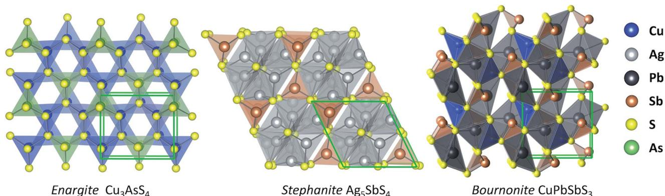
Fig. 2 Illustrations of the crystal structures of candidate solar minerals: enargite (space group *Pmn2*<sub>1</sub>), stephanite (space group *Cmc2*<sub>1</sub>), and bournonite (space group *Pmn2*<sub>1</sub>).
