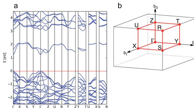
Fig. 3 Calculated electronic band structure of enargite ( $\text{Cu}_3\text{AsS}_4$ ) (a) and the reciprocal space  $k$ -path for the structure determined by the Aflow-online utility<sup>74</sup> (b).
