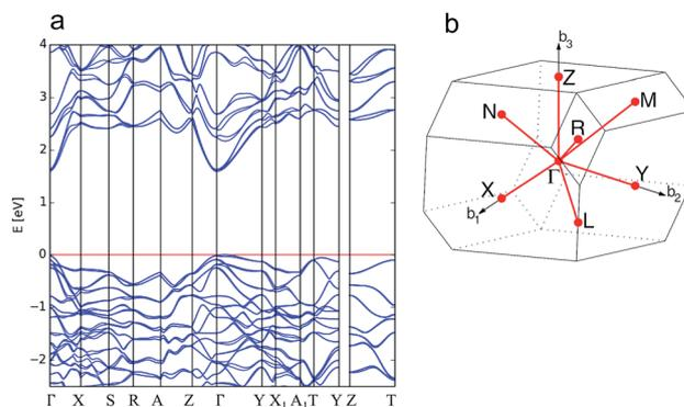
Fig. 8 Calculated electronic band structure of stephanite ( $\text{Ag}_5\text{SbS}_4$ ) (a) and the reciprocal space  $k$ -path for the structure determined by the Aflow-online utility<sup>74</sup> (b).
