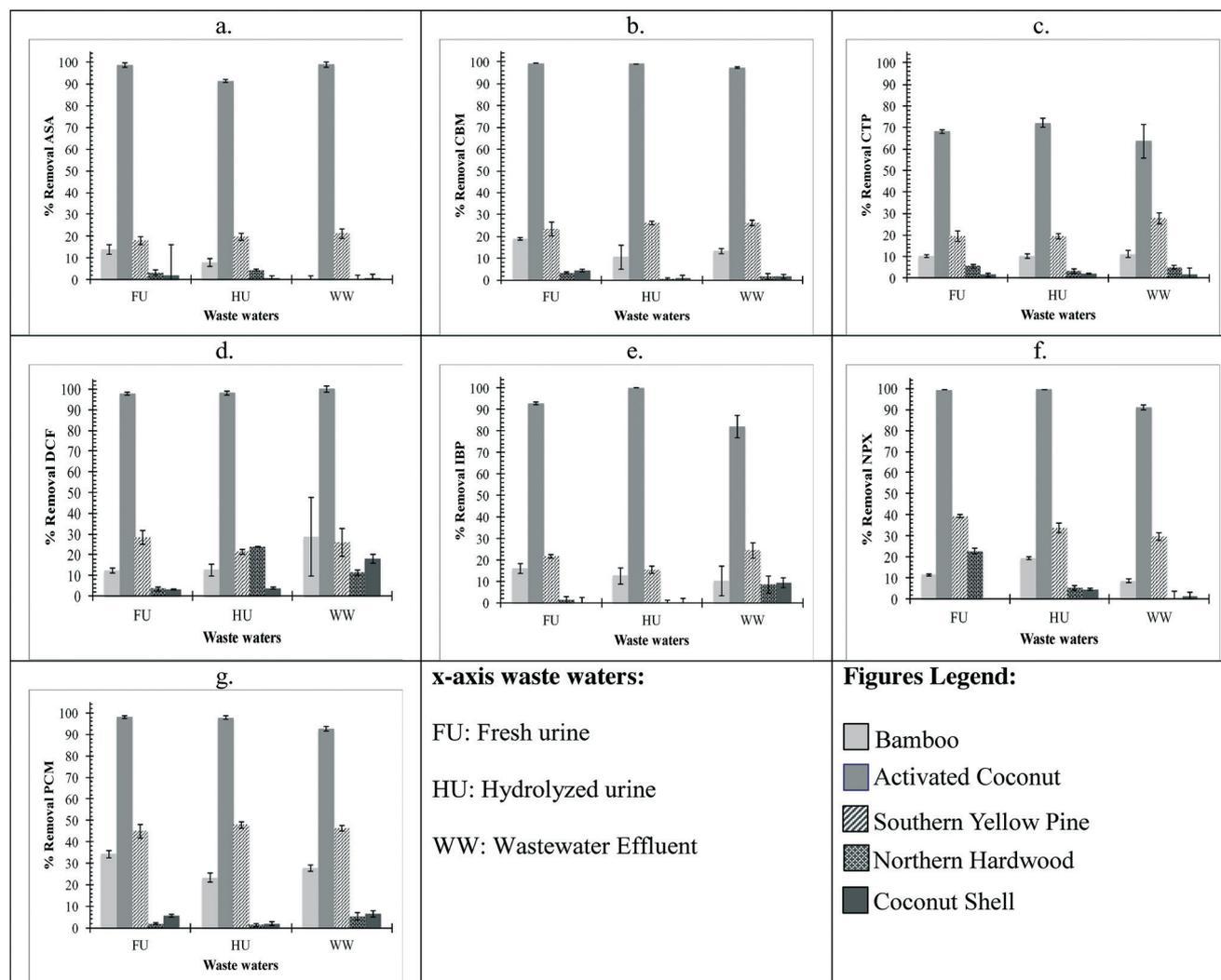
Fig. 2 Pharmaceutical removal by biochar at  $0.8 \text{ g L}^{-1}$  dose and 300 rpm for 24 h ( $C_0 = 0.2 \text{ mmol L}^{-1}$ ). Pharmaceuticals: a. ASA, b. CBM, c. CTP, d. DCF, e. IBP, f. NPX, and g. PCM. Error bars indicate one standard deviation for triplicate samples.
