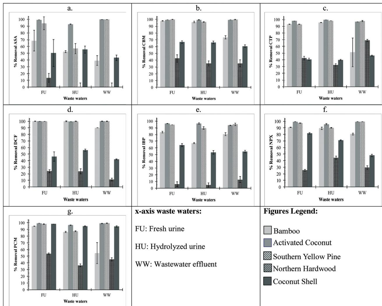
Fig. 1 Pharmaceutical removal by biochar at  $40 \text{ g L}^{-1}$  dose and 300 rpm for 24 h ( $C_0 = 0.2 \text{ mmol L}^{-1}$ ). Pharmaceuticals: a. ASA, b. CBM, c. CTP, d. DCF, e. IBP, f. NPX, and g. PCM. Error bars indicate one standard deviation for triplicate samples.
