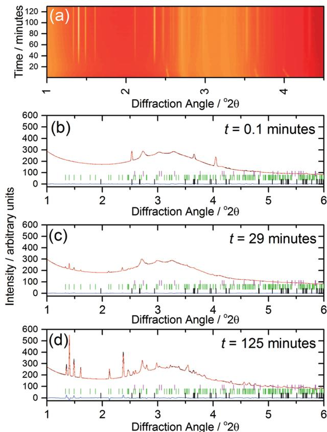
Fig. 7 (a) Heatmap of *in situ* data during crystallisation of (2) and (b–d) final profile fits obtained at three different times. In (b)–(d) the observed data are in black, the final Pawley fit in red and the difference curve in blue, while the pink, green and black ticks are Bragg peak positions for the unit cells of PEEK, (2) and 1,4-benzenedicarboxylic acid, respectively.
