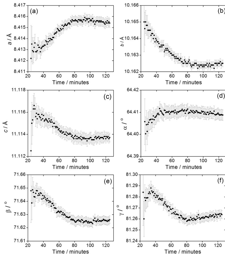
**Fig. 9** Evolution of triclinic lattice parameters (a)  $a$ , (b)  $b$ , (c)  $c$ , (d)  $\alpha$ , (e)  $\beta$  and (f)  $\gamma$  during the crystallisation of (2). Error bars are standard deviations from the Pawley fitting.
