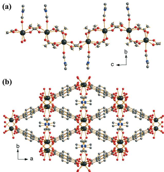
Fig. 1 Structure of (1): (a) fragment of infinite chain running along *c* and (b) view along *c* showing diamond shaped channels containing Yb-coordinated DMF (one orientation drawn). Large dark grey atoms are Yb, small grey atoms are C, red atoms are O and blue are N. Hydrogen atoms are omitted for clarity and broken-off bonds represent connections to neighbouring atoms.
